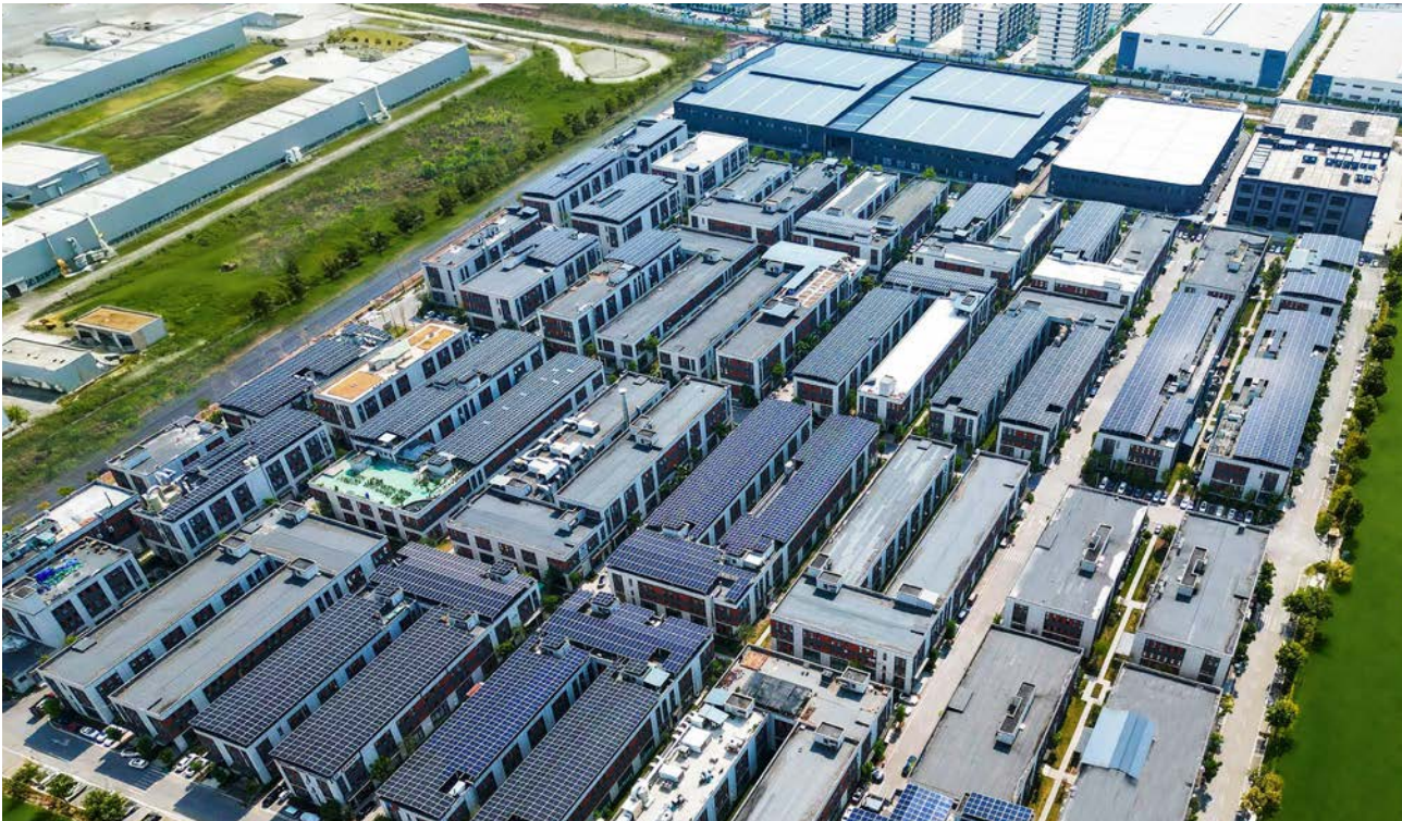
📍 Chongqing High-tech Park | Installed Capacity: 5.2MW | 1st-Year Generation: 6GWh
